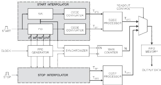
Figure 2. Block diagram of the time counter
