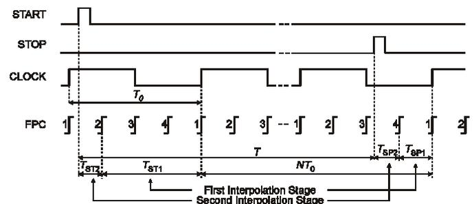
Figure 1. Two-stage interpolation method
