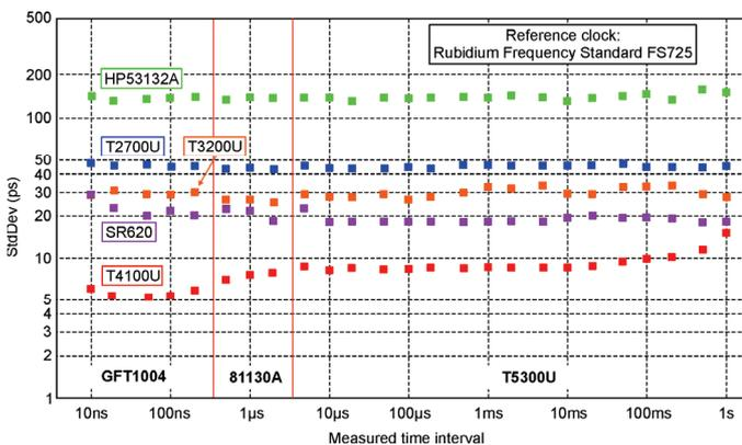
Figure 8. Comparison of the precision (standard measurement uncertainty) of successive versions of our time counter (T2700U with a single coding line, T3200U with a double coding line and T4100U with multiple coding lines) and selected commercial time counters (HP53132A, Hewlett-Packard and SR620, Stanford Research Systems)
