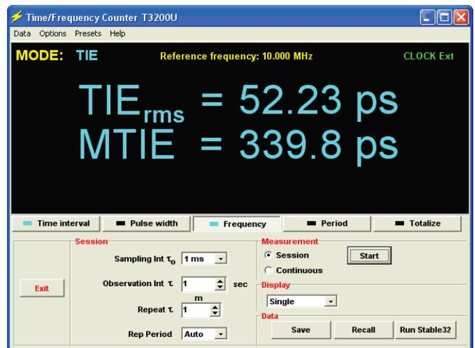
Figure 6. Virtual front panel of the counter operating in the TIE mode
