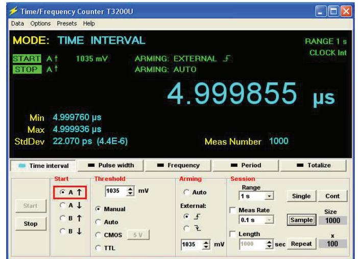
Figure 4. Example of the virtual front panel of the counter operating in the Time Interval mode
