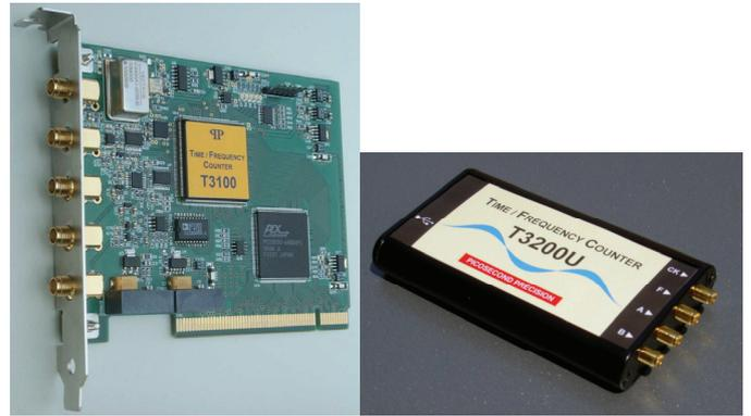
Figure 3. External view of the counter board with PCI interface and the counter module with USB interface
