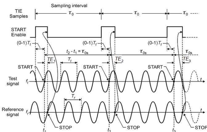
Figure 5. Measurement of Time Interval Error
