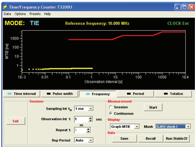
Figure 7. Graph MTIE( $\tau$ ) with limit mask (G.812 clock 1)
